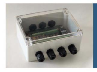
The digital I/O box is used with the EXAConnecT controller. It allows 24 volt I/O signals from up to seven tools to be sent to a PLC. The box is IP 54 (NEMA 12) rated for dust and moisture resistance.
