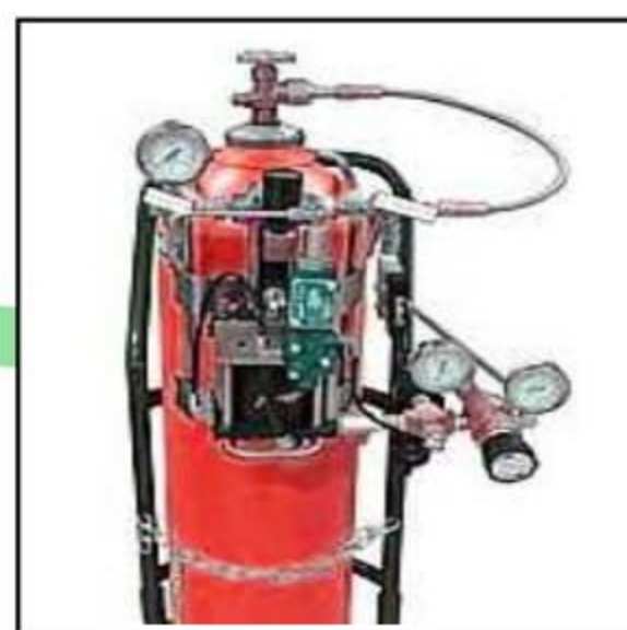
Transfer of fluids and filling up of high pressures tank.
